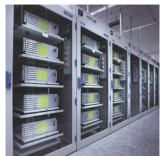
36-hour run-in test at 40 °C
